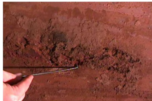
Figure 18. Internal corrosion at the rupture site
