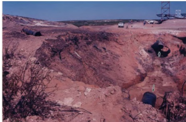
Figure 16. The crater left after the rupture
